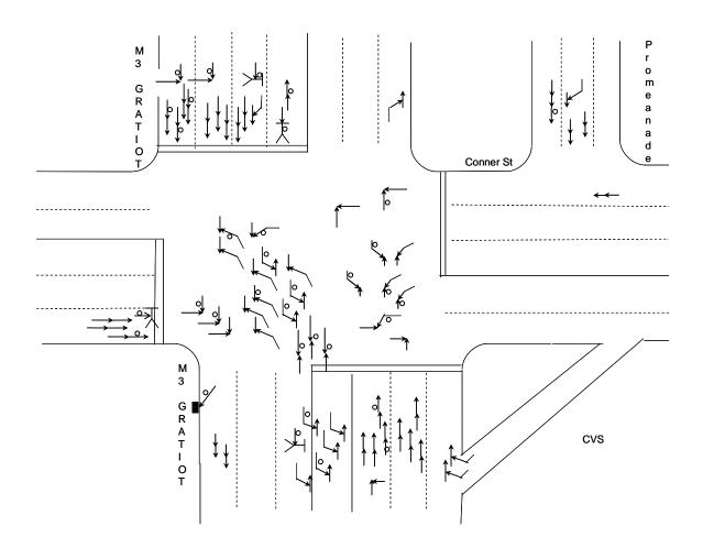
Fig 5.21-A: Collision Diagram
