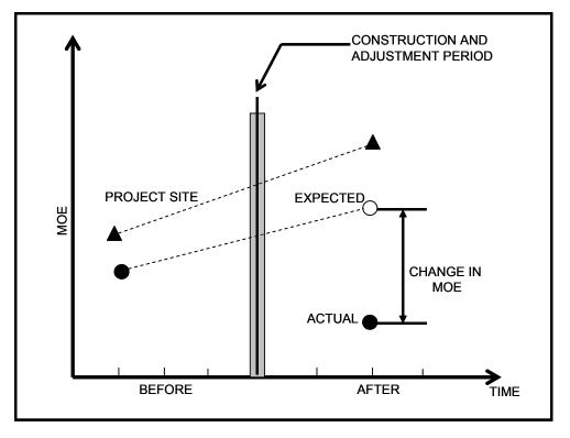
Fig. 2.3 Experimental Design a Before and After Study with Control Site Method (Source Ref: 23)
