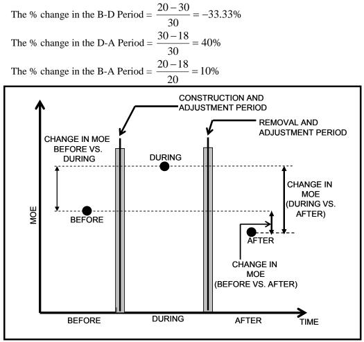
Fig. 2.5 Experimental Design of a Before-During-After Method (Source Ref: 23)
