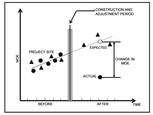
Fig. 2.4 Experimental Design of a Before and After Study with Control Sites with Trend Analysis (Source Ref: 23)
