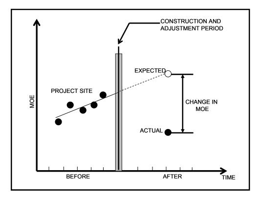
Fig. 2.2 Experimental Design of a Before and After Study with Trend Analysis. (Source Ref: 23)
