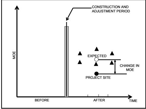
Fig. 2.6 Experimental Design of a Comparative Parallel Study Method (Source Ref: 23)
