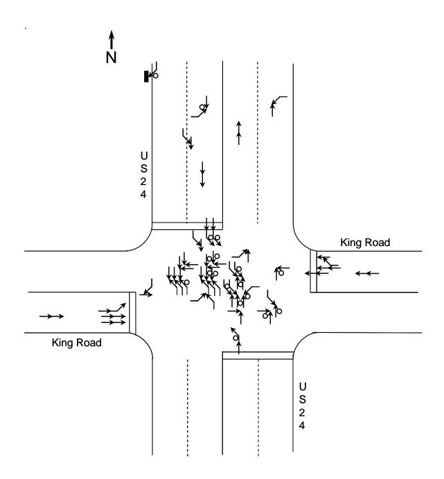
Figure 5.12: Collision Diagram of US24 and King Road
