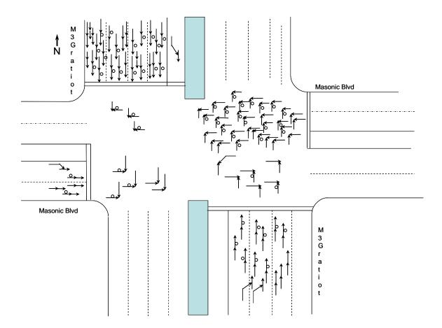
Fig 5.4: Collision Diagram of M-3 Gratiot and Masonic Blvd.
