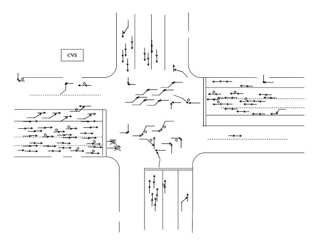
Fig 5.30-A: Collision Diagram
